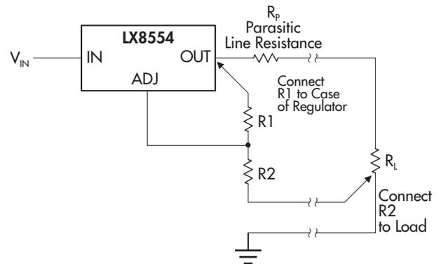
FIGURE 3 — CONNECTIONS FOR BEST LOAD REGULATION
