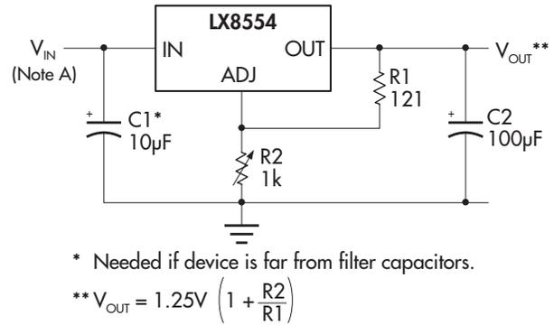
FIGURE 5 — 1.2V - 8V ADJUSTABLE REGULATOR
