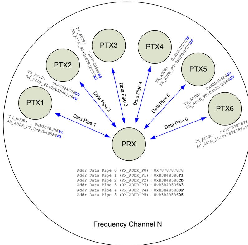
Figure 15. Example of data pipe addressing in MultiCeiver™
