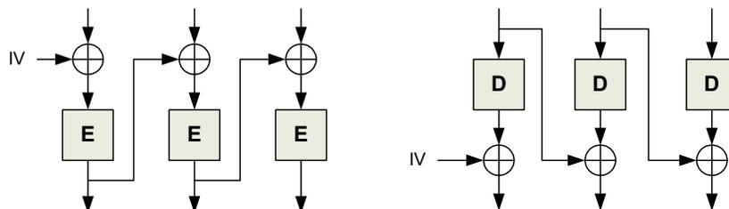
Figure 42. CBC – Cipher Block Chaining mode
