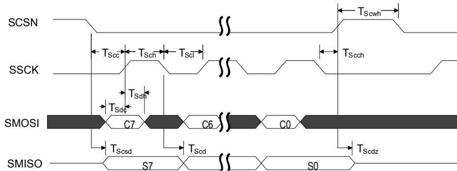
Figure 49. Slave SPI timing diagram
