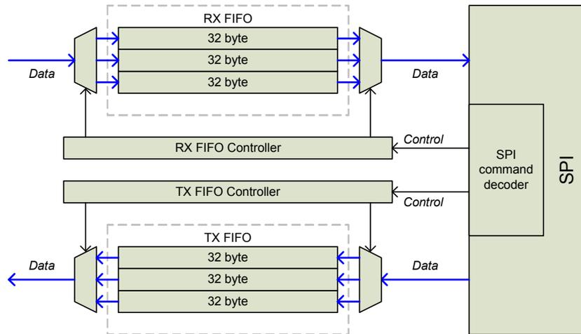
Figure 27. FIFO (RX and TX) block diagram
