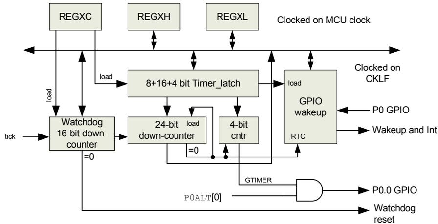
Figure 72. Block diagram of wakeup and watchdog functions
