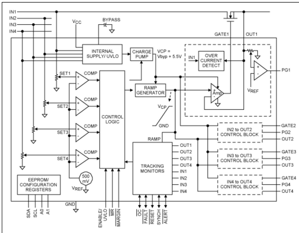
Figure 5. A programmable quad voltage tracker (MAX6876).
