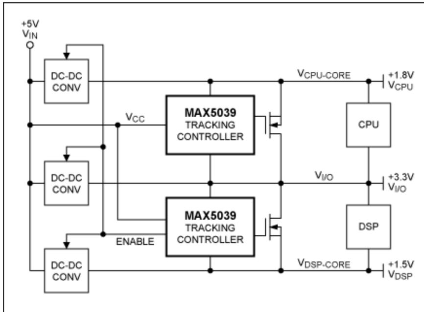
Figure 4. Multivoltage systems require multiple tracking controllers.
