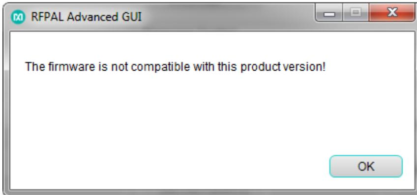
This error message is displayed when trying to load the SC1894 firmware into the SC1905 chip or the SC1905 firmware into the SC1894 chip.
