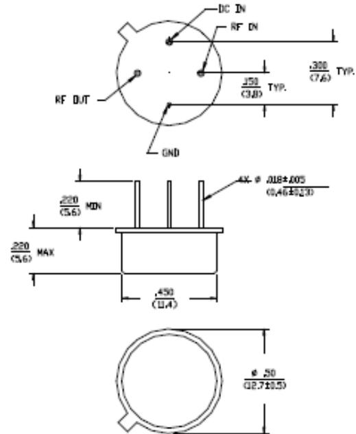
Dimensions in  $\text{\O}$  are in mm
