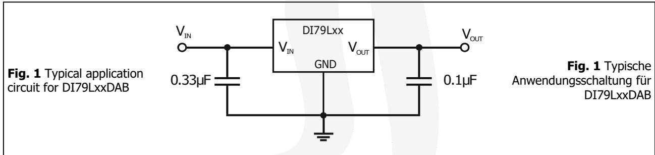
**Fig. 1** Typical application circuit for DI79LxxDAB
