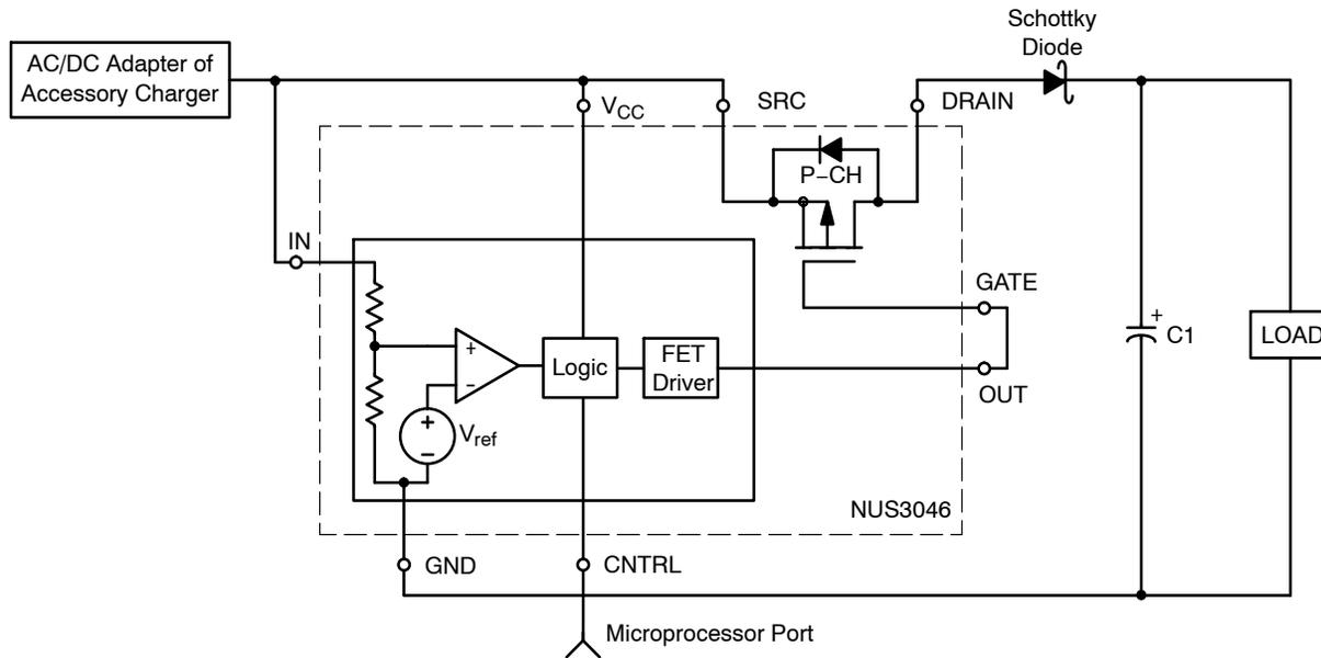
Figure 1. Simplified Schematic
