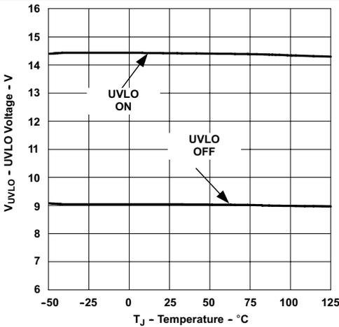
Figure 9. Undervoltage Lockout vs Temperature
