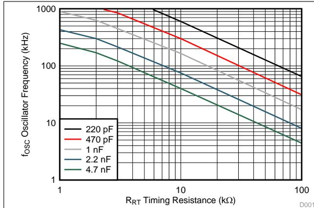
Figure 1. Oscillator Frequency vs Timing Resistance and Capacitance
