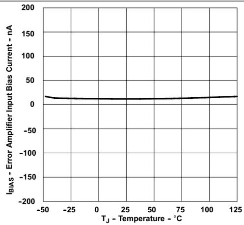
Figure 8. Error Amplifier Input Bias Current vs Temperature
