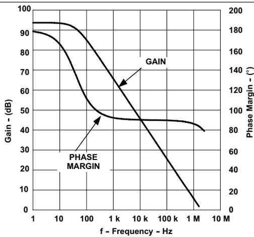
Figure 3. Error Amplifier Frequency Response
