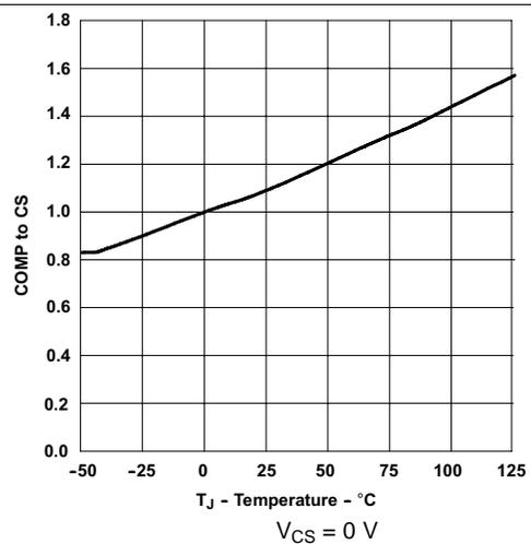
Figure 4. COMP to CS Offset Voltage vs Temperature
