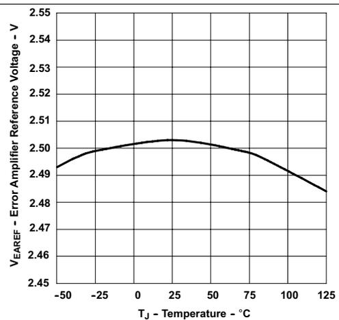
Figure 6. Error Amplifier Reference Voltage vs Temperature
