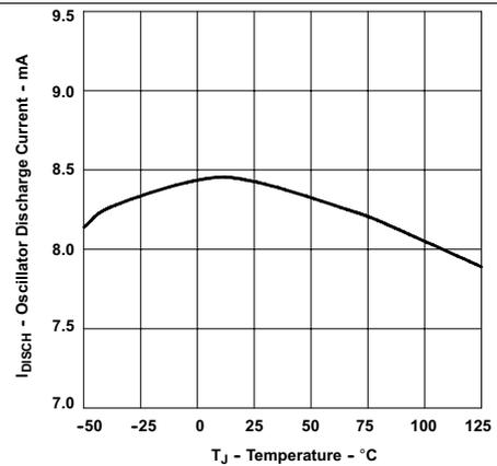
Figure 2. Oscillator Discharge Current vs Temperature
