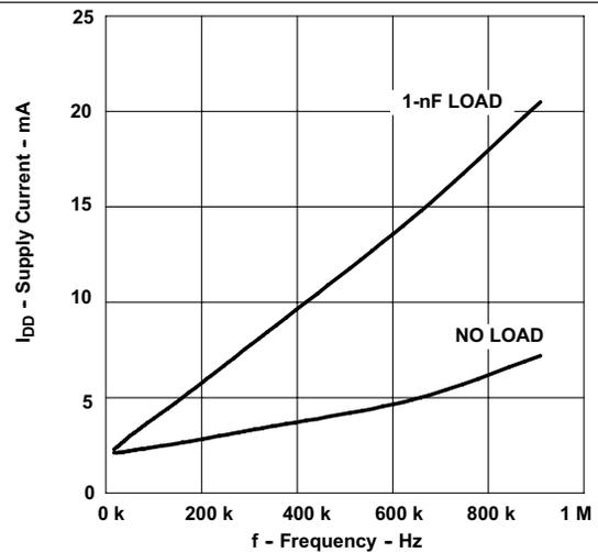
Figure 12. Supply Current vs Oscillator Frequency
