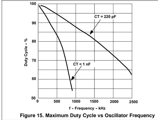
Figure 15. Maximum Duty Cycle vs Oscillator Frequency
