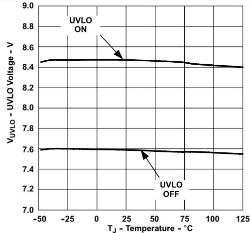
Figure 10. Undervoltage Lockout vs Temperature
