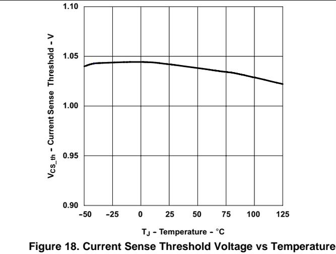
Figure 18. Current Sense Threshold Voltage vs Temperature
