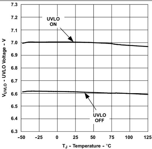
Figure 11. Undervoltage Lockout vs Temperature
