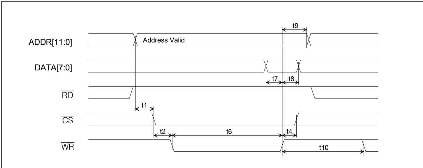
**Figure 15-3. Motorola Bus Read Timing (BTS = 1)**
