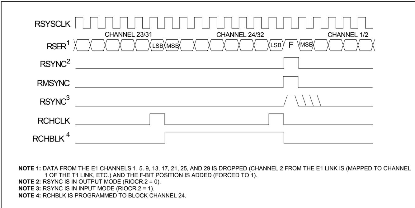
**Figure 13-18. E1 Receive-Side 2.048MHz Boundary Timing (Elastic Store Enabled)**
