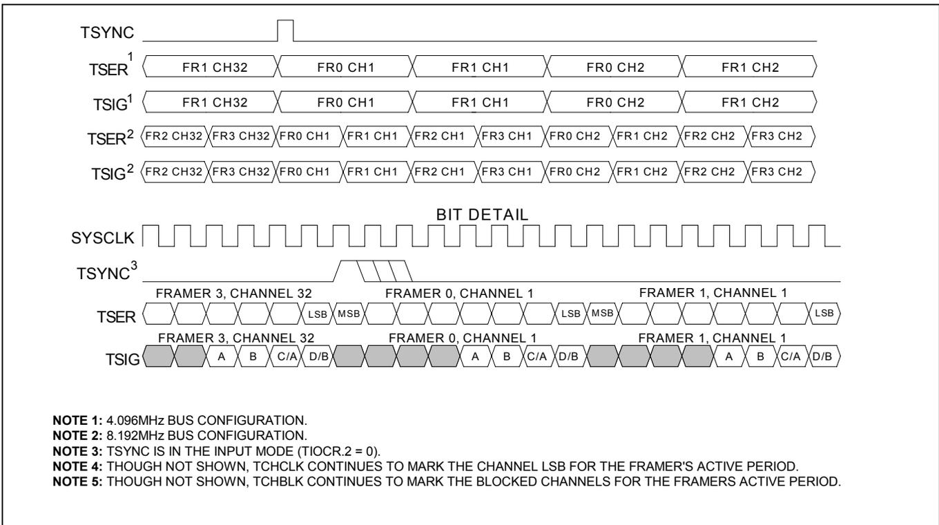
**Figure 13-14. T1 Transmit Interleave Bus Operation, FRAME Mode**
