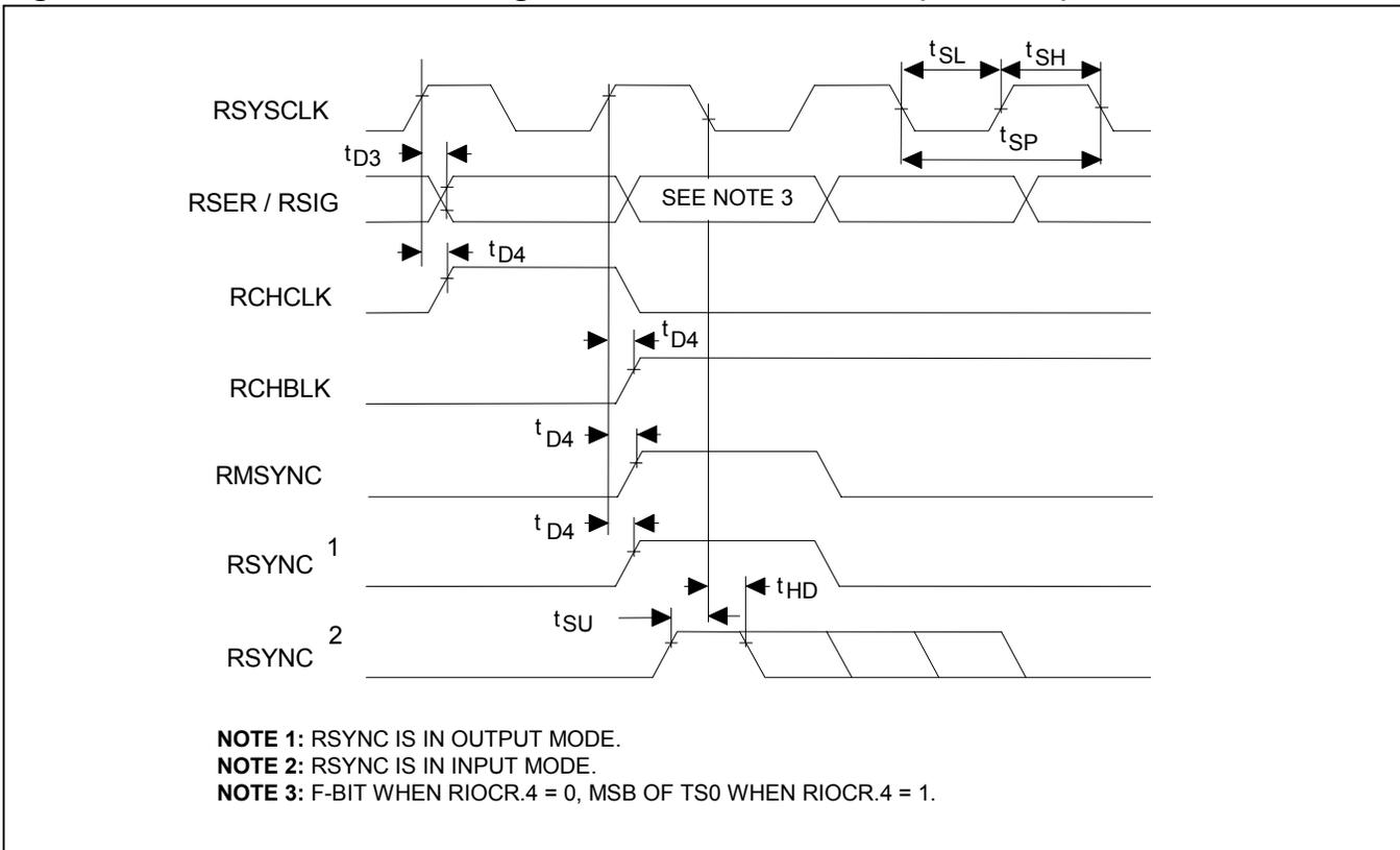
**Figure 15-7. Receive Framer Timing—Line Side**
