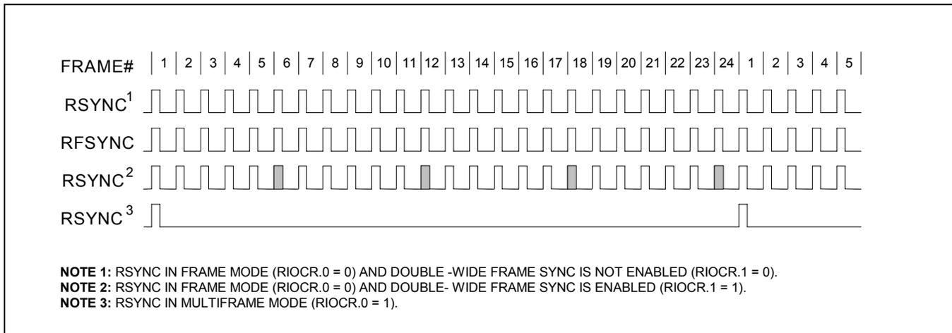
**Figure 13-3. T1 Receive-Side Boundary Timing (Elastic Store Disabled)**
