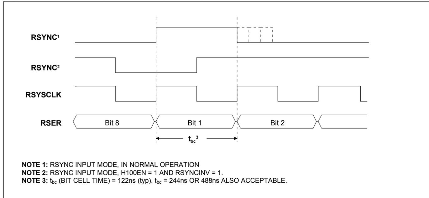
Figure 8-2. TSSYNC Input in H.100 (CT Bus) Mode
