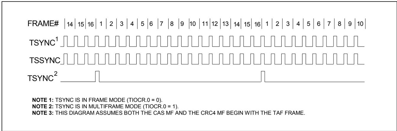
**Figure 13-20. E1 Transmit-Side Boundary Timing (Elastic Store Disabled)**
