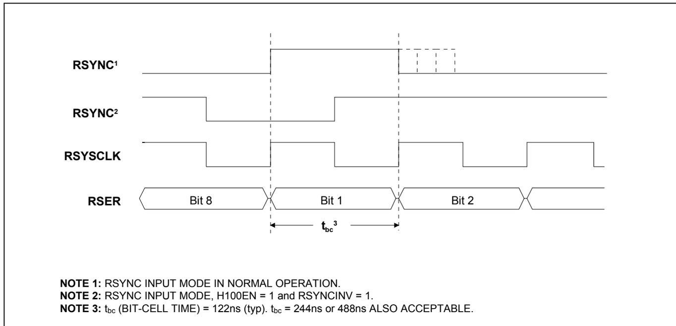
Figure 10-2. TSSYNC Input in H.100 (CT Bus) Mode
