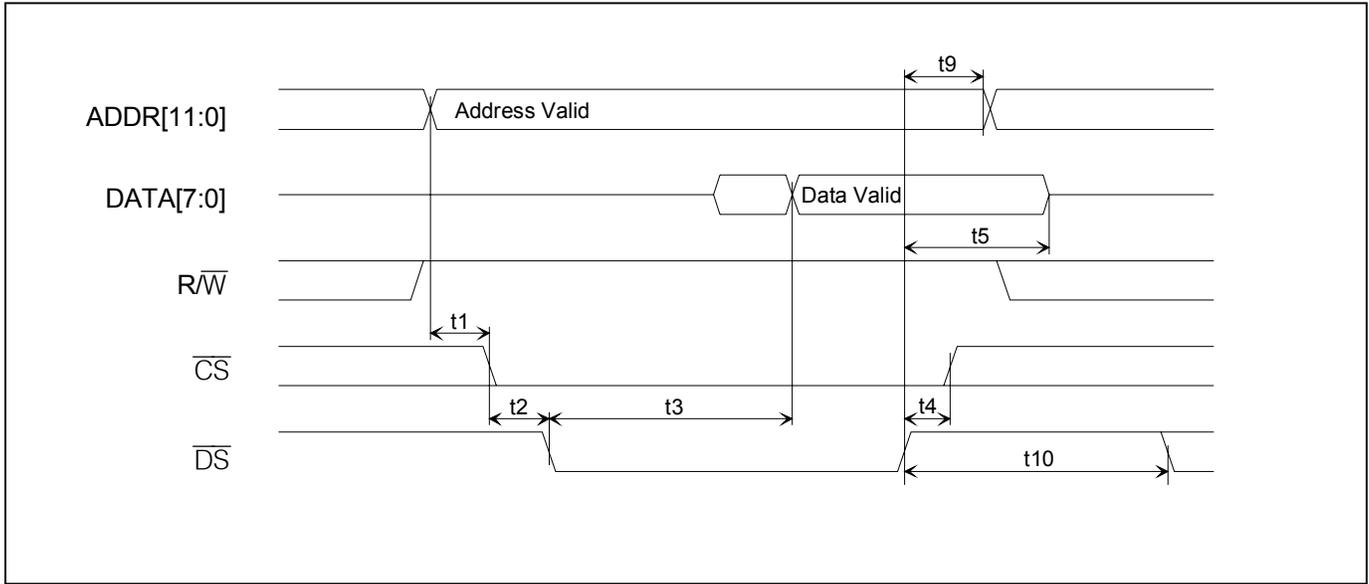
**Figure 15-4. Motorola Bus Write Timing (BTS = 1)**
