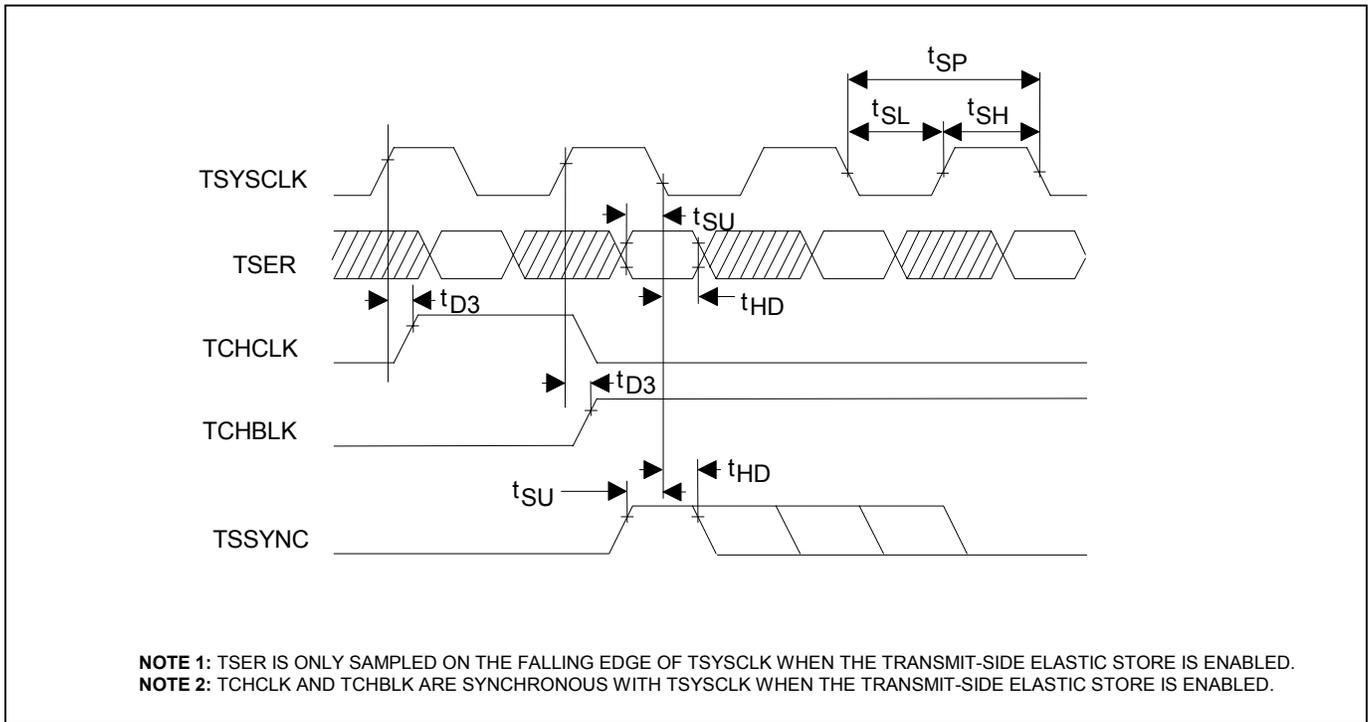
**Figure 15-10. Transmit Formatter Timing—Line Side**
