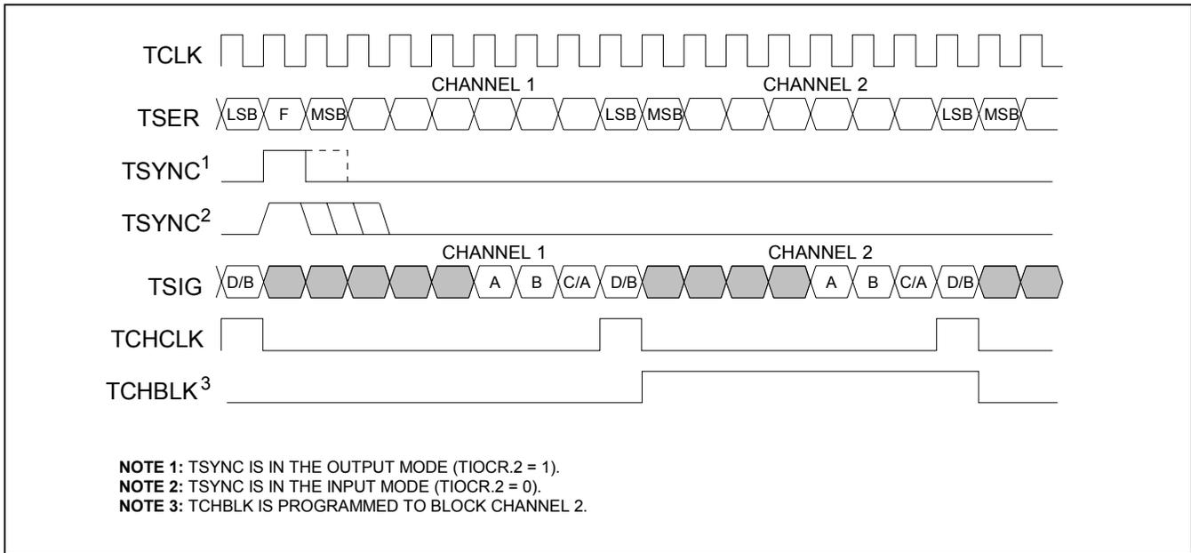
**Figure 13-11. T1 Transmit-Side 1.544MHz Boundary Timing (Elastic Store Enabled)**
