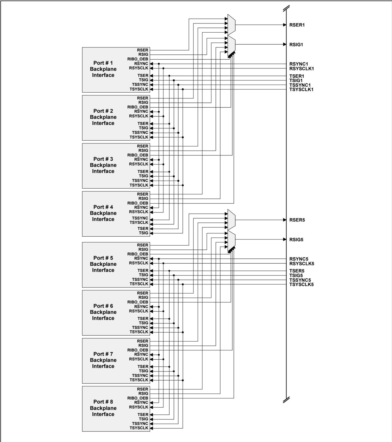
Figure 7-3. Internal IBO Multiplexer Equivalent Circuit—16.394MHz
