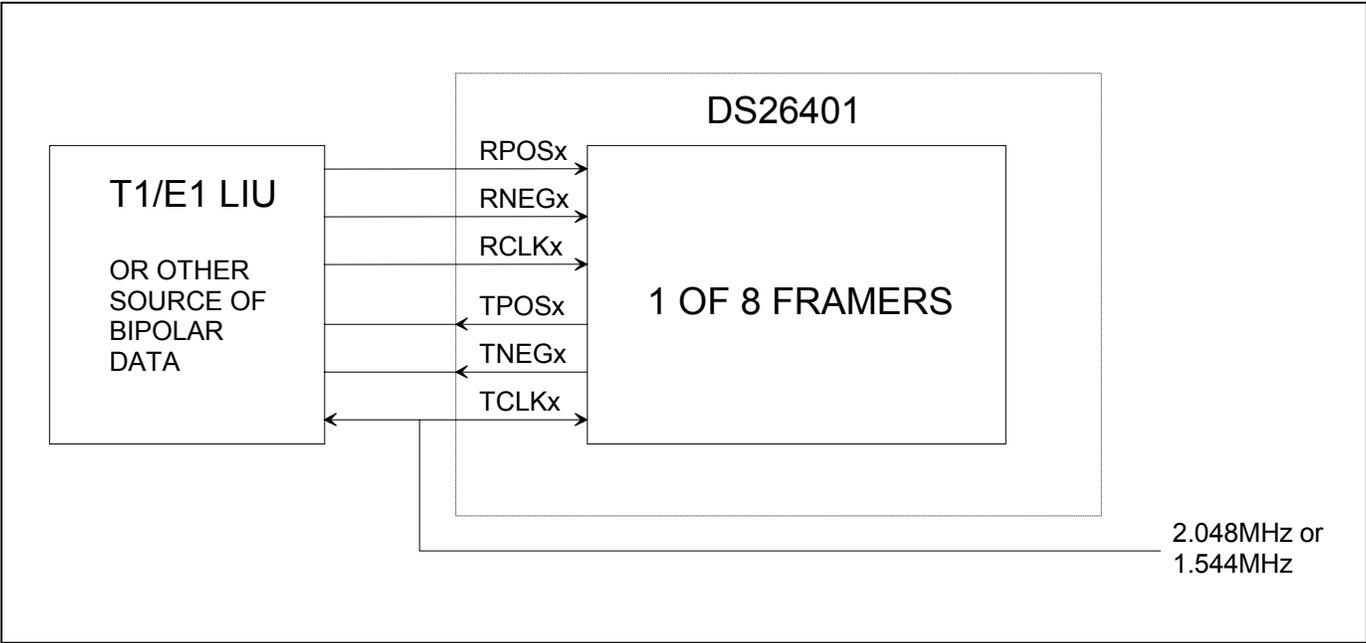
Figure 3-4. Typical NRZ Network-Side Interface to Framers
