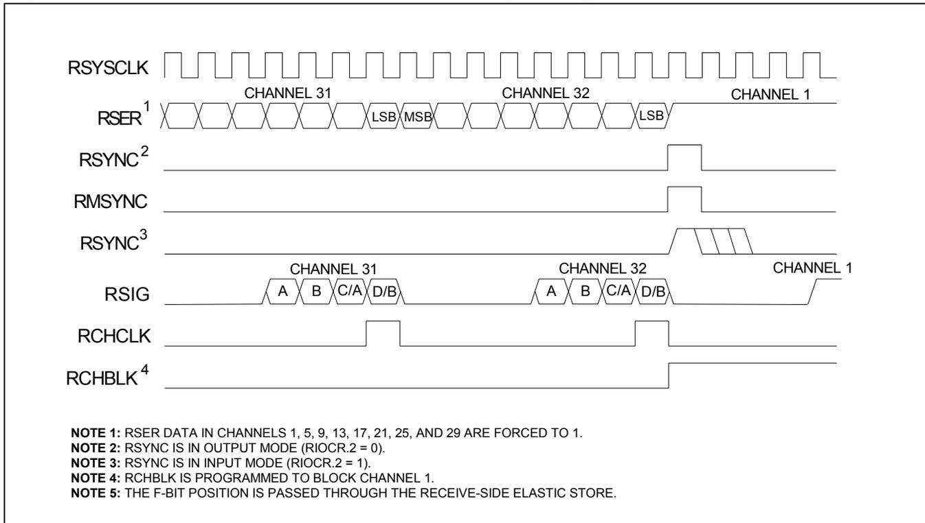
**Figure 13-6. T1 Receive-Side Interleave Bus Operation, BYTE Mode**
