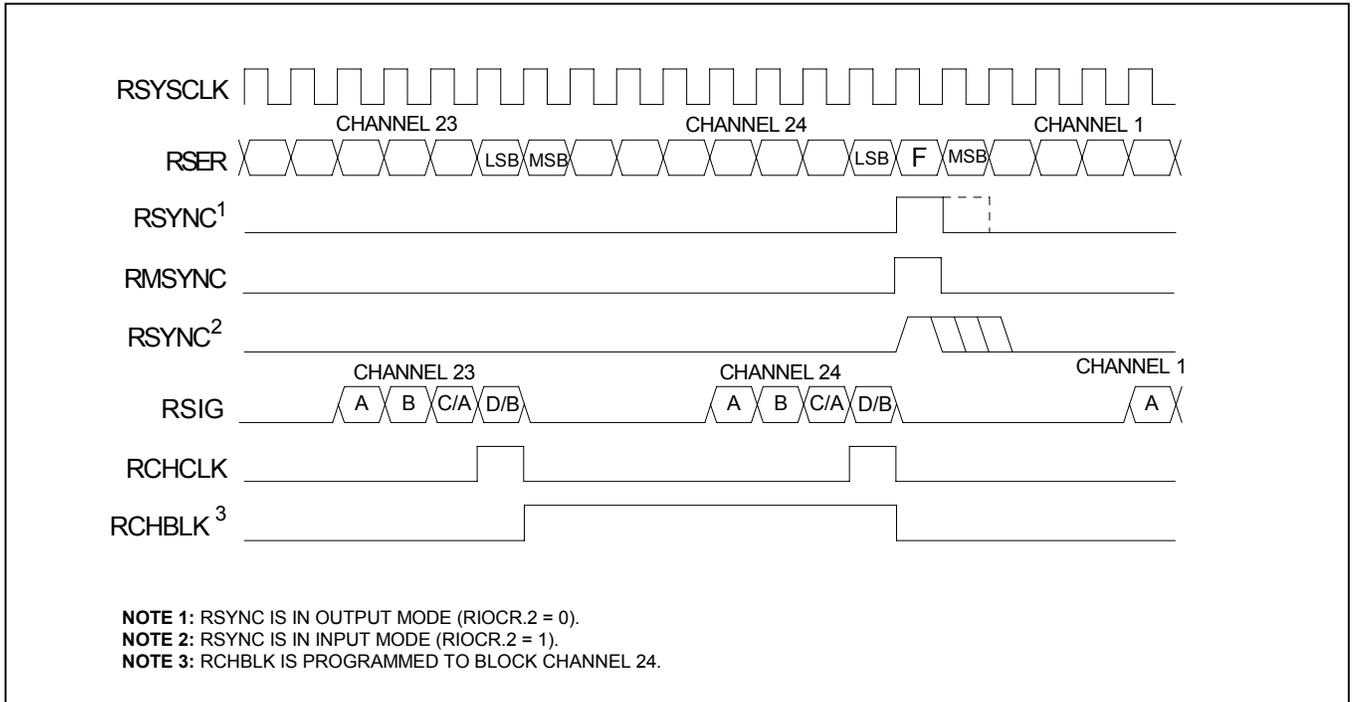
**Figure 13-5. T1 Receive-Side 2.048MHz Boundary Timing (Elastic Store Enabled)**
