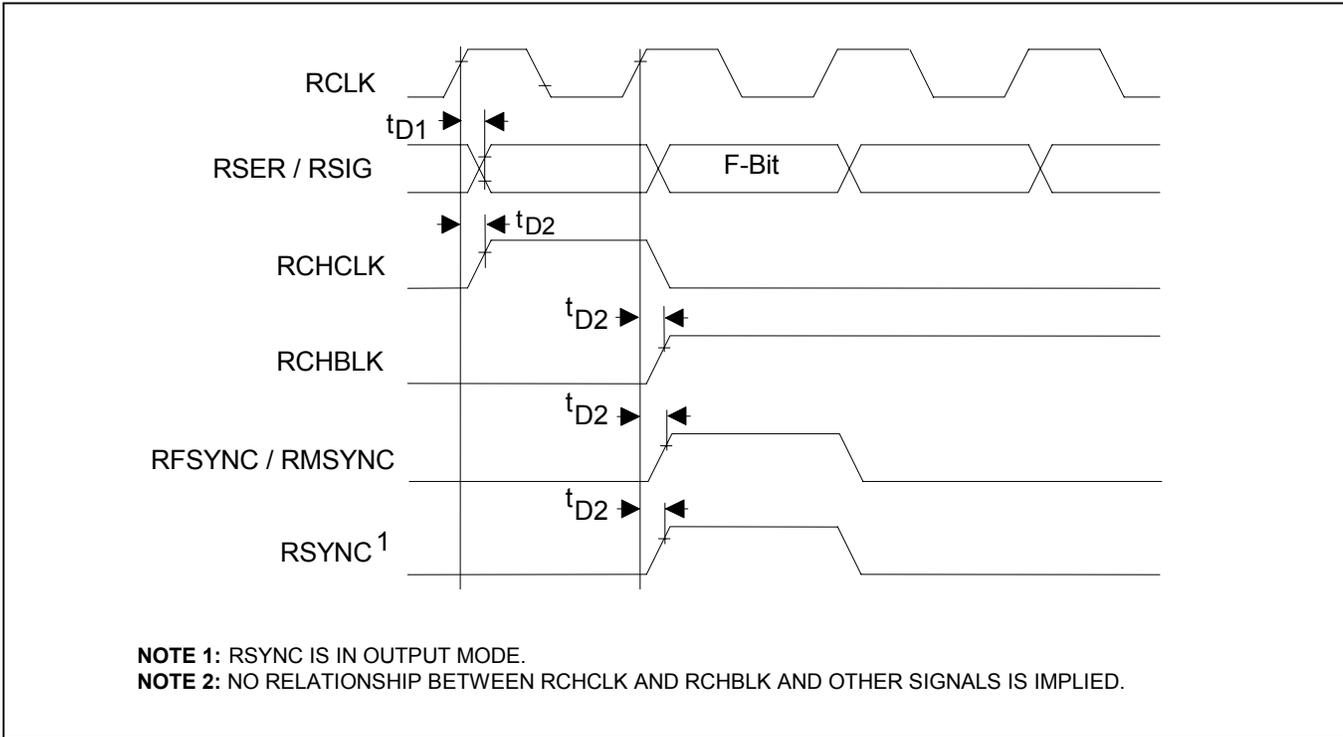
**Figure 15-6. Receive-Side Timing—Elastic Store Enabled (T1 Mode)**
