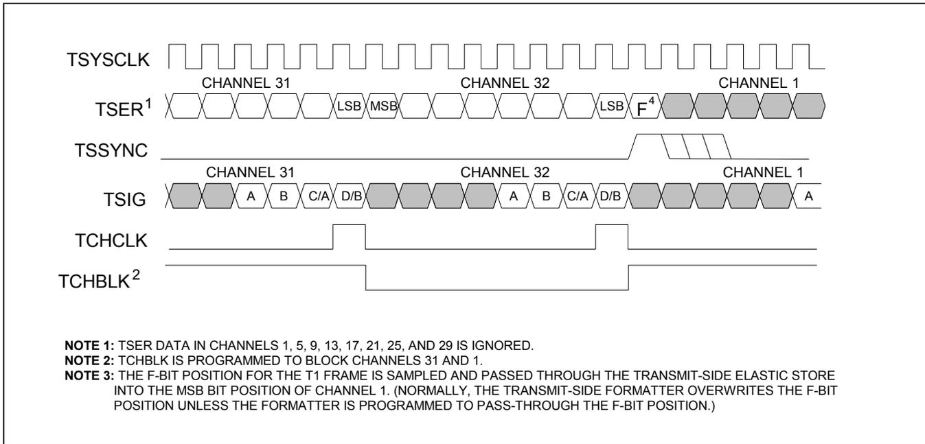
**Figure 13-13. T1 Transmit-Side Interleave Bus Operation, BYTE Mode**
