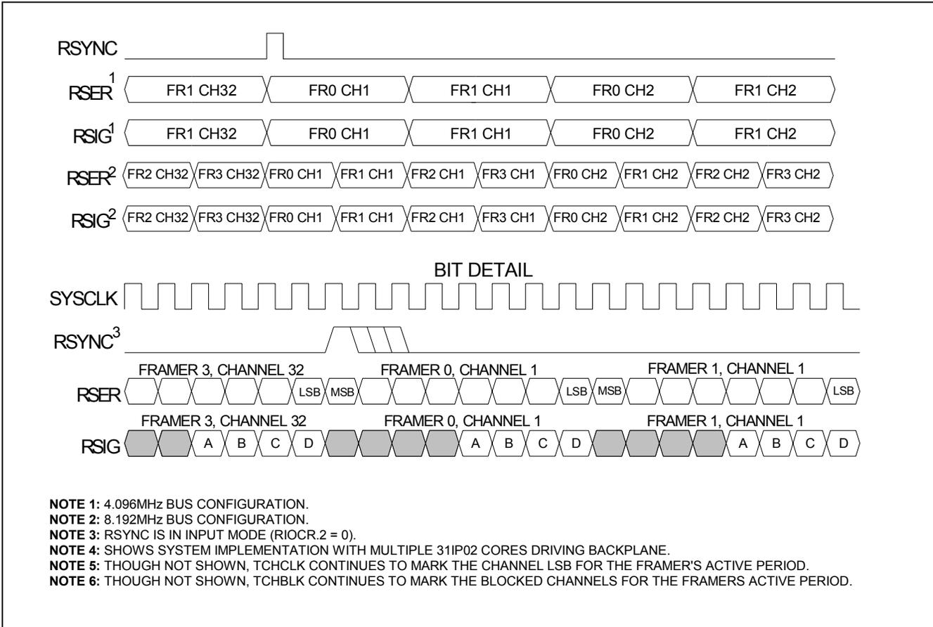
**Figure 13-7. T1 Receive-Side Interleave Bus Operation, FRAME Mode**
