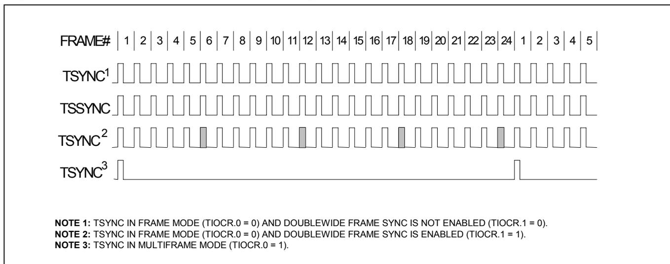
**Figure 13-10. T1 Transmit-Side Boundary Timing (Elastic Store Disabled)**
