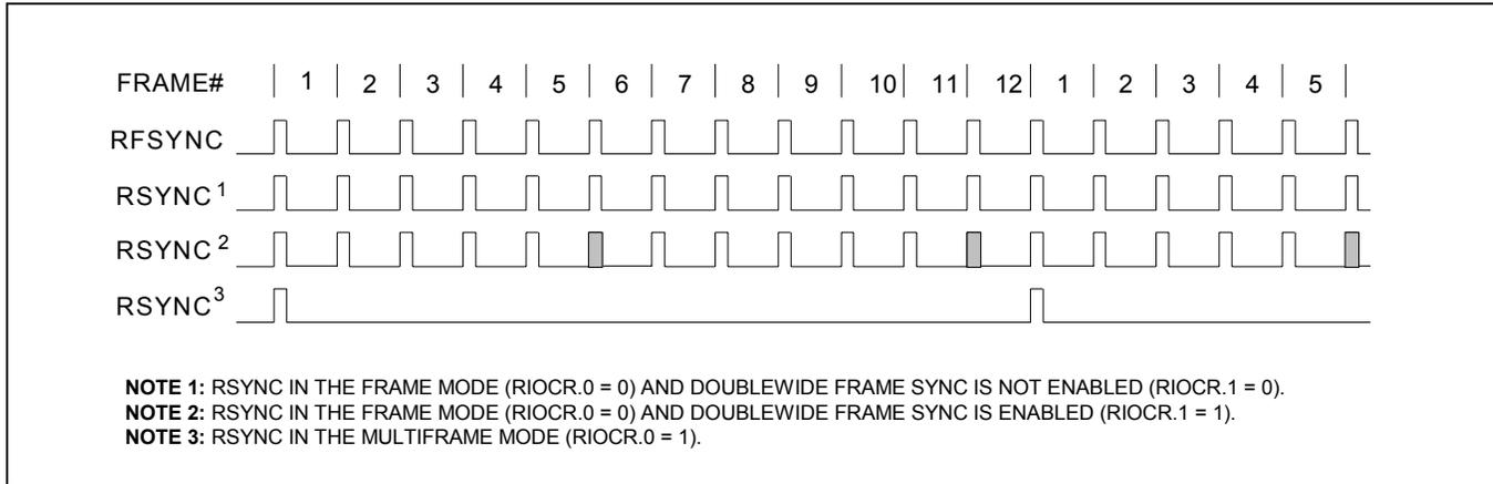
**Figure 13-2. T1 Receive-Side ESF Timing**
