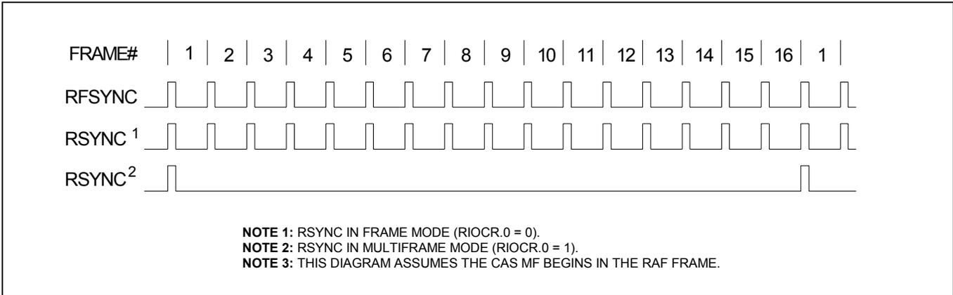
Figure 13-16. E1 Receive-Side Boundary Timing (Elastic Store Disabled)
