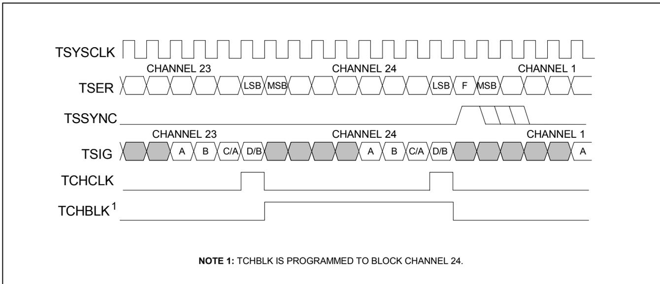
**Figure 13-12. T1 Transmit-Side 2.048MHz Boundary Timing (Elastic Store Enabled)**
