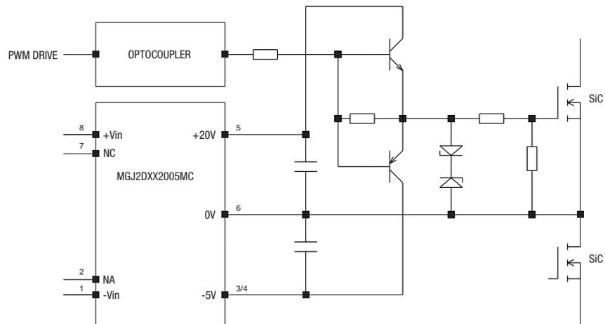
MGJ2 DC-DC CONNECTIONS FOR DRIVING MOSFET DEVICES
