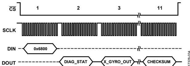
Figure 42. Burst Read Sequence with BURST\_SEL = 0
