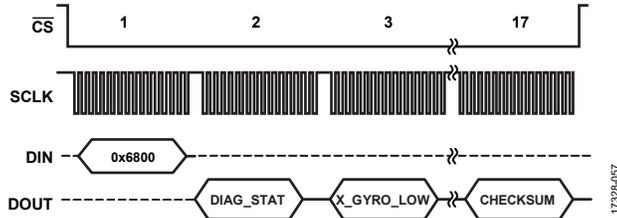
Figure 44. Burst Read Sequence with BURST\_SEL = 0
