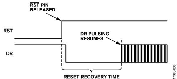
Figure 38. Data Ready Response During Reset ( $\overline{RST} = 0$ ) Recovery
