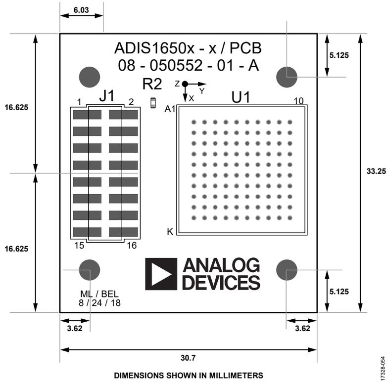
Figure 64. Top View of the ADIS16505 Breakout Board
