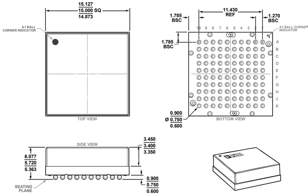
Figure 66. 100-Ball Ball Grid Array Module [BGA]
