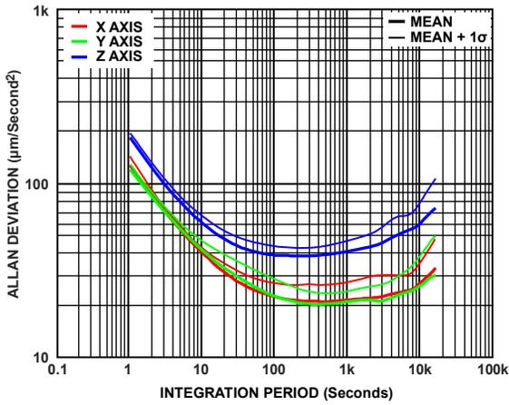
Figure 23. Accelerometer Allan Deviation,  $T_c = 25^\circ\text{C}$
