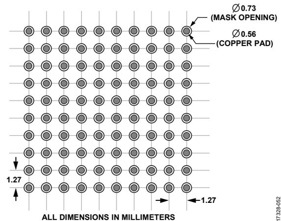
Figure 62. Recommend PCB Pattern, Solder Mask Defined Pads
