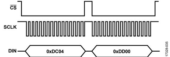
Figure 46. SPI Sequence for Writing 0x0004 to FILT\_CTRL
