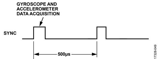
Figure 29. Sync Output Signal, Register MSC\_CTRL, Bits[3:2] = 11
