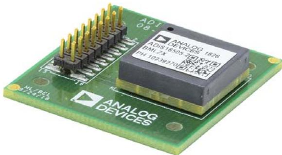
Figure 63. ADIS16505-2 Breakout Board
