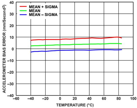
Figure 24. Accelerometer Bias Error vs. Temperature, All Axes
