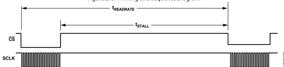
Figure 3. Stall Time and Data Rate Timing Diagram
