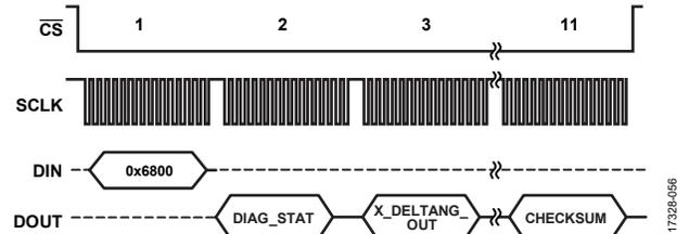
Figure 43. Burst Read Sequence with BURST\_SEL = 1
