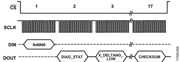
Figure 45. Burst Read Sequence with BURST\_SEL = 1
